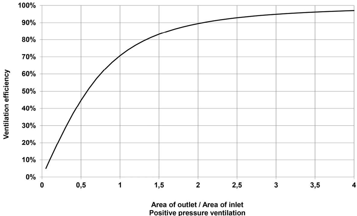
Figure 3: Relation between inlet area and outlet area when using positive pressure ventilation.
