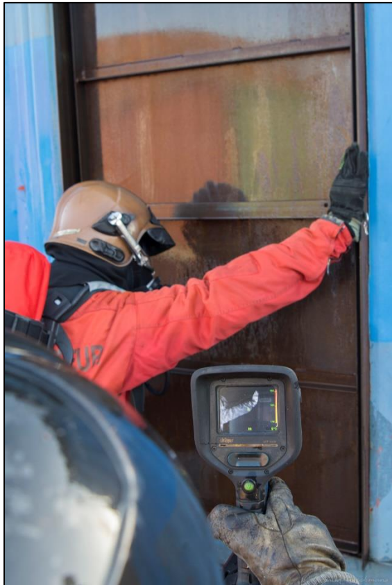
figure 3 The nozzle man is searching for hinges to determine whether it is an inward or an outward opening door. (Photo: German Berckmans)
