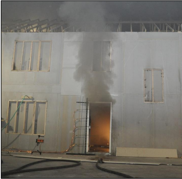
figure 4 The smoke is exiting through the upper end of the door while the rest of the door opening is used for air that is flowing in. The fresh air will cause the fire to grow faster. (Photo: Steve Kerber – Underwriters Laboratories)
