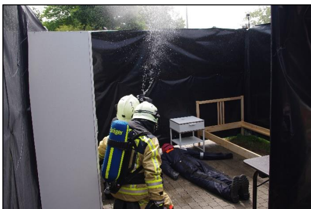
figure 4 Searching with a hose takes longer and air consumption is higher. (Photo: Steve De Blauwe)
