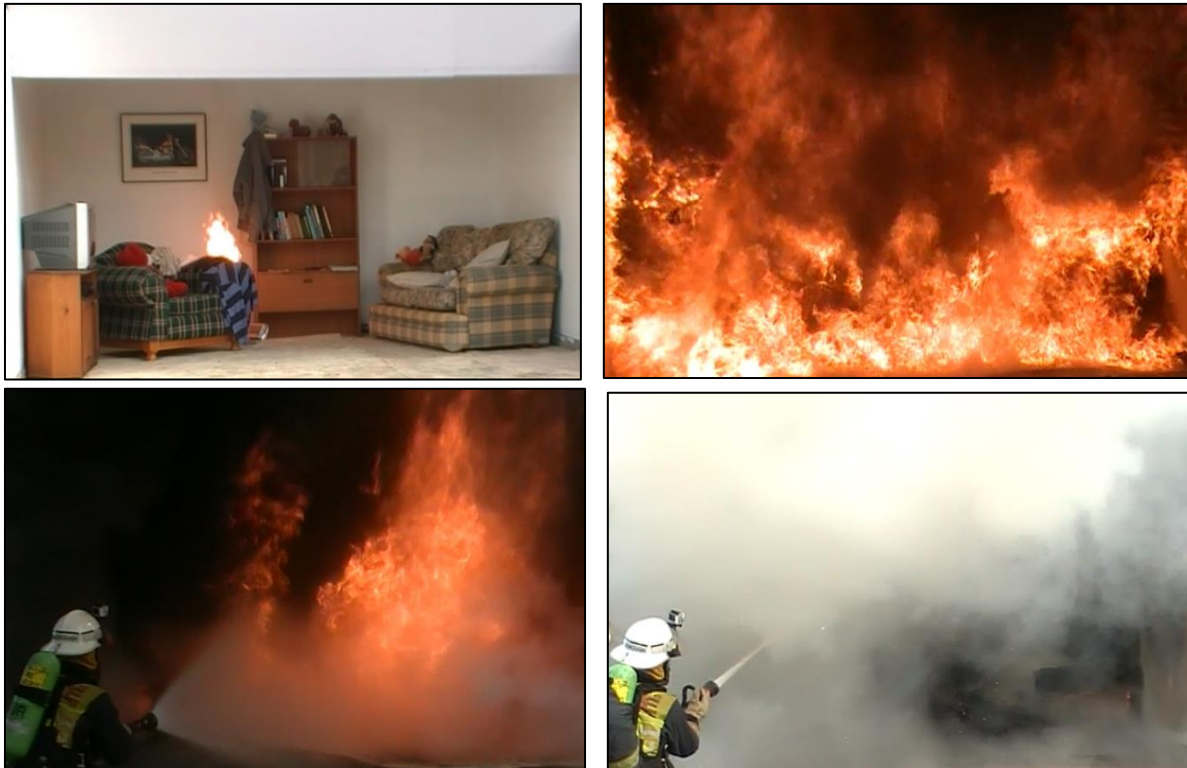
figure 6 The development of a beginning fire (upper left) to fully developed (upper right). Next the fully developed fire is knocked down using an indirect attack. That indirect attack can be seen in the bottom left image. After knockdown, the firefighter has to switch to a direct attack to fully extinguish the fire. (Photo: New South Wales Fire & Rescue Service)
