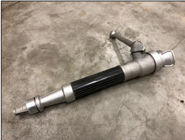
figure 2 The “standardized” nozzle (Photo: Warre St-Germain)
