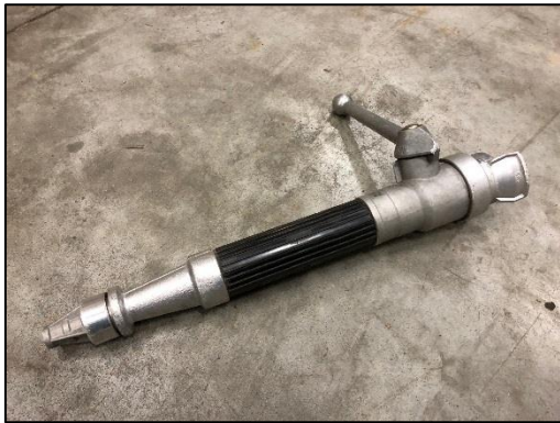
figure 4 Nowadays there are modern variants of this old nozzle. In the US, this type of nozzle is called "Smooth bore". (Photo: Warre St-Germain)
