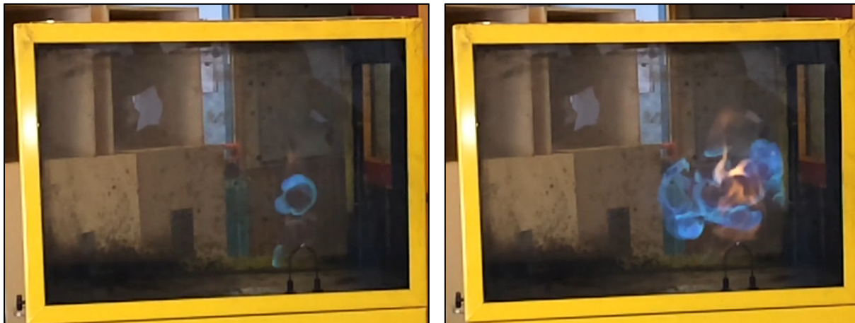
Figure 1 Ignition of a mixture of gas and air. On the left-hand picture, ignition has just occurred. The flame front is moving in a circular way into all directions. The right-hand picture shows an increase of the volume of flames. (Photo's: Karel Lambert)
