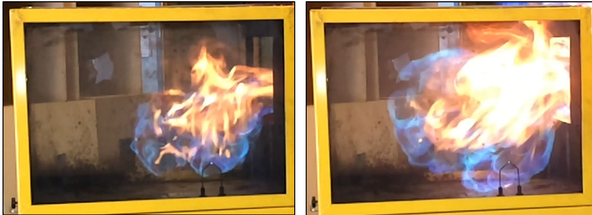
Figure 2 These photos show the rest of the reaction process illustrated in Figure 1. The left-hand photo shows the flame spreading further. This is also shown in the right-hand photo. That way, the flames are spreading along the entire volume in which the mixture is inside the flammable range. (Photo's: Karel Lambert)
