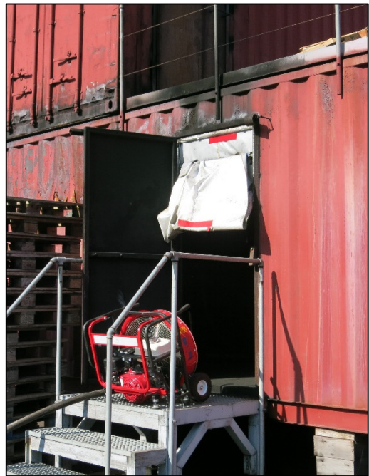
Figuur 6 The smoke stopper closes the upper half of the door opening. The backflow caused by the fan is limited. The fan can be placed closer to the door. (Picture: Michael Reick)
