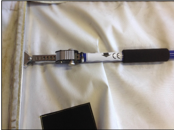
Figure 4 Close up of the positioning mechanism of the smoke stopper. By pressing the clip the rod can be adjusted. Subsequently turning the bar in the direction of the arrow, adds tension which holds the device in place (Photo: Karel Lambert)
