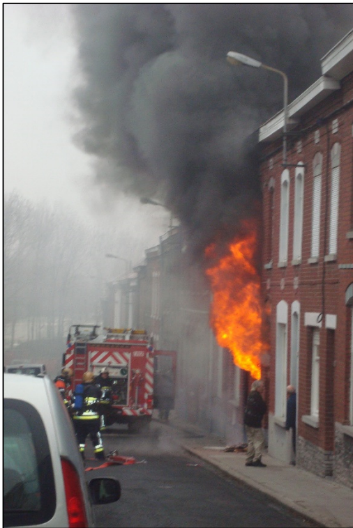
Figure 3 A fully developed fire in a room should be put out using under 500 litres of water. (Photo: Moeskroen Fire Department)
