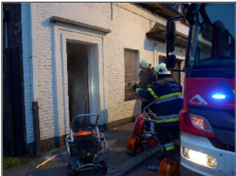
Figure 4 Positioning of two positive pressure fans in V-formation. (Photo: Frank Meurisse)
