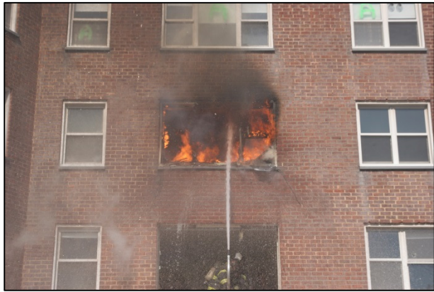
Figure 5 Use of the floor below nozzle in order to flow water into the burning apartment under wind driven conditions. (Photo: NIST)
