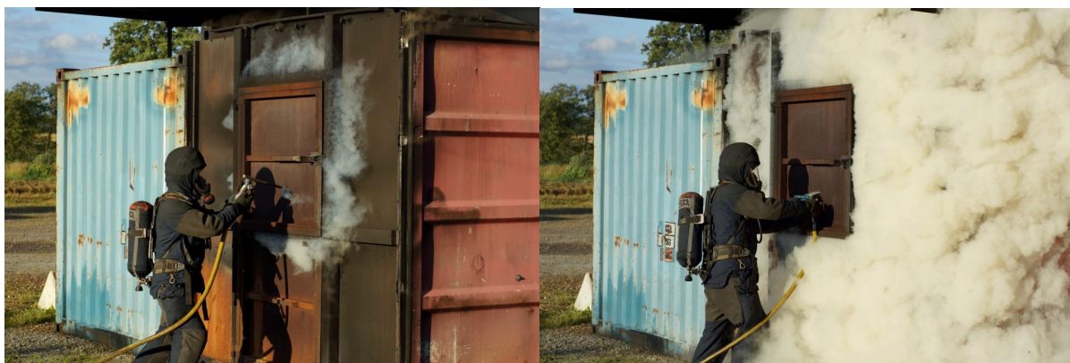
Figure 3 Applying a piercing nozzle in a pre-backdraft situation. The water being flowed in will create a cooling effect. Large amounts of steam are also formed that inert the room. (Photo: Lars Ågerstrand)
