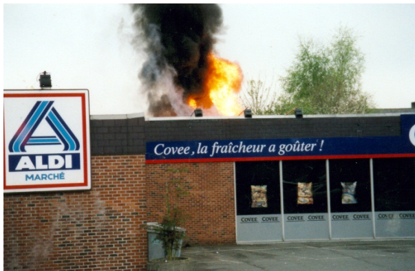
Figure 6 The photograph shows three shades from left to right : pyrolysis gas, smoke gas and flames. The clarity of the flames indicates auto-ignition of exiting smoke gas. (Photo: Benoît Amans)
