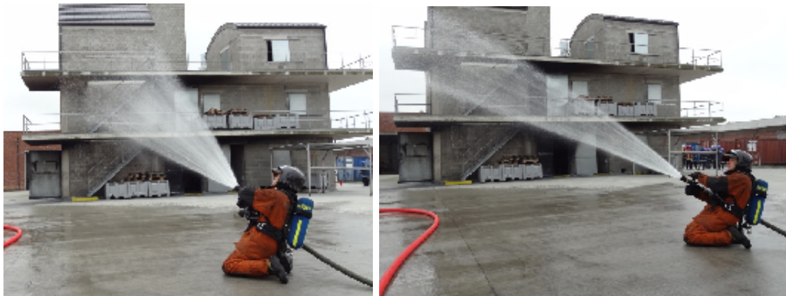
Figure 1.3 & 1.4 In the left image a short pulse is shown. The angle of the nozzle in regard to the ground level is 45°. The angle of the water cone ranges from 40° to 60°. The photograph on the right shows a long pulse. The angle between the nozzle and the ground level is approximately 30° and the angle of the cone is also 30°. (Photos: Geert Vandamme)
