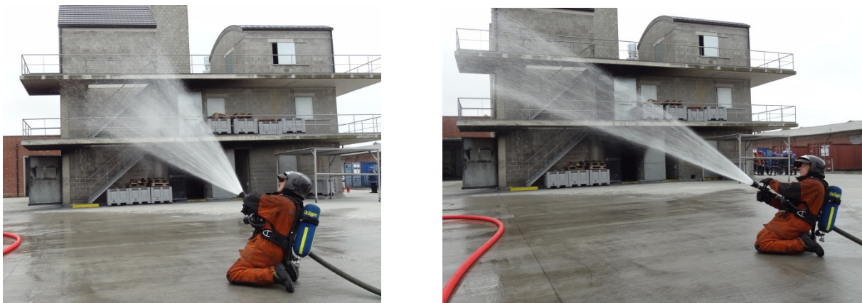
Figure 1.3 & 1.4 In the left image a short pulse is shown. The angle of the nozzle in regard to the ground level is 45°. The angle of the water cone ranges from 40° to 60°. The photograph on the right shows a long pulse. The angle between the nozzle and the ground level is approximately 30° and the angle of the cone is also 30°. (Photos: Geert Vandamme)
