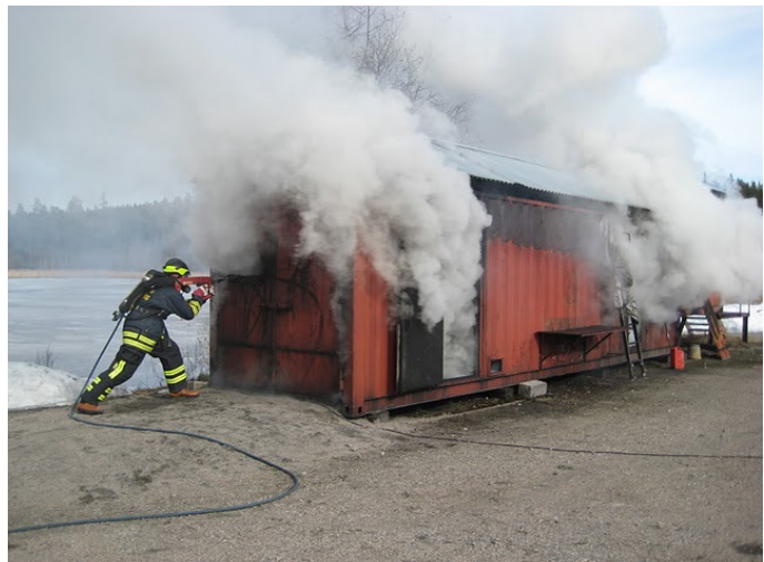
Fig 12.4 The Cobra in action on a training site. The fire gases are rendered completely inert and are cooled. (Picture by: Willem Nater)
