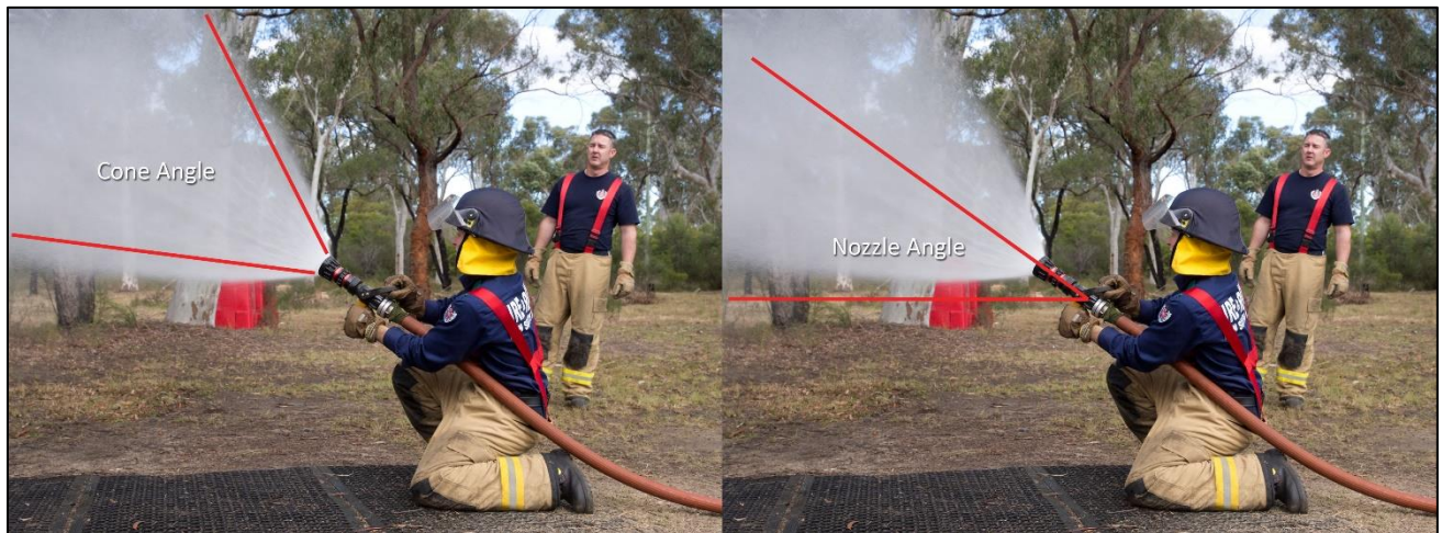
Image 3. Cone angle vs nozzle angle.
