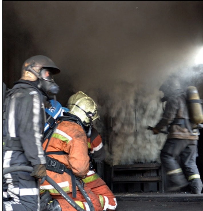
Figure 7 Firefighters during an exercise in the backdraft cell. The firefighters are in front of a closed door. The door separates the compartment from the oven where a stack of pallets is burning. The fire has become ventilation controlled. Due to the overpressure inside, pyrolysis gases are pushed through the cracks that surround the door. (Picture: Erik Etienne)
