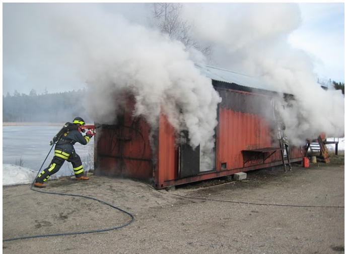
Figure 19 Application of the cobra at a fully developed fire during a training course with the cobra cutting extinguisher. (Picture: Willem Nater [40])
