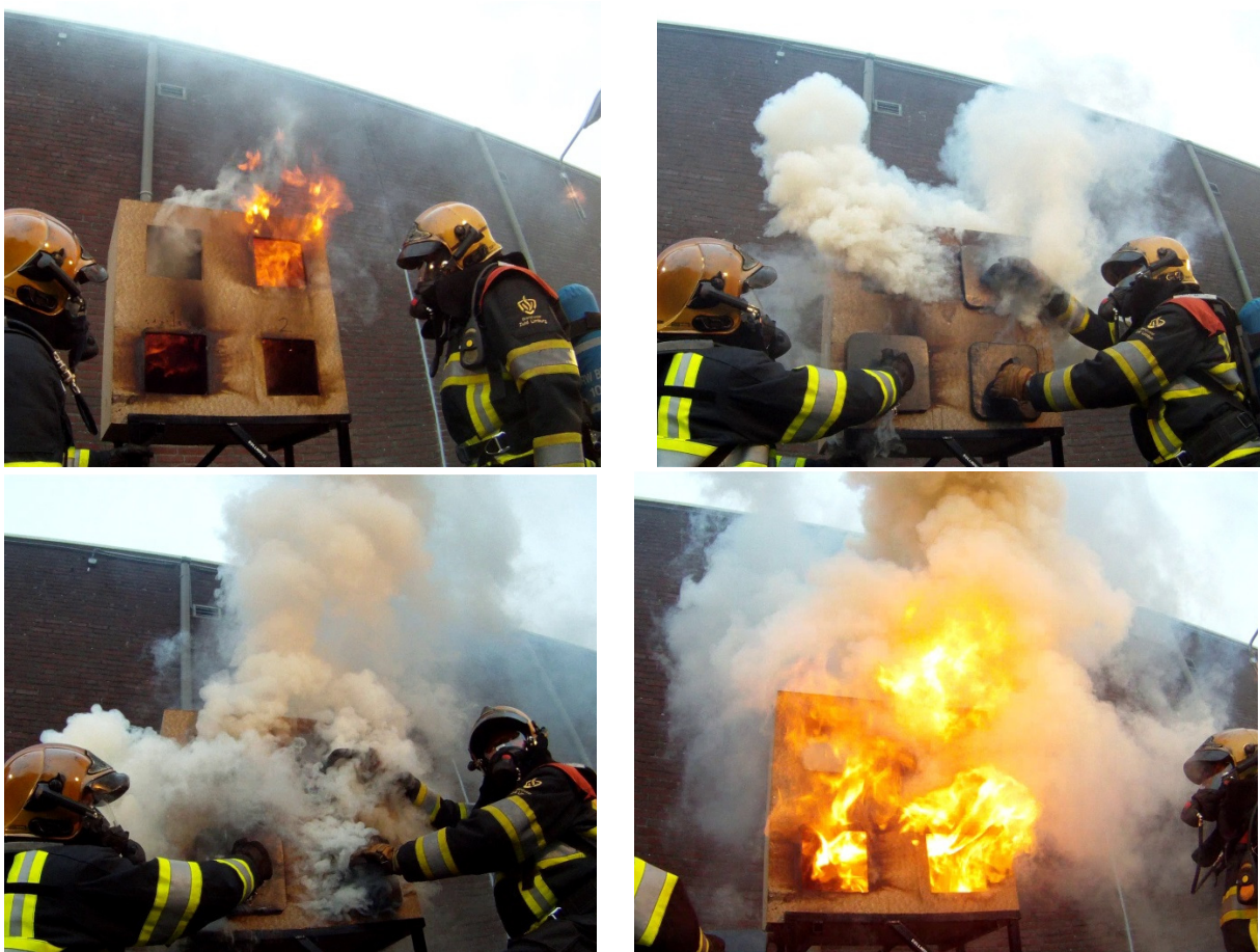
Figure 5 Sequences of a four compartment doll's house demonstration. The fire is fully developed in the upper right compartment in the first picture. Three openings are closed in the second picture. The fourth room doesn't connect with the other rooms. The fire generates lots of pyrolysis gases (picture bottom left). When the doors to the three rooms are opened, a backdraft like phenomenon occurs (Picture: CFBT-NL)
