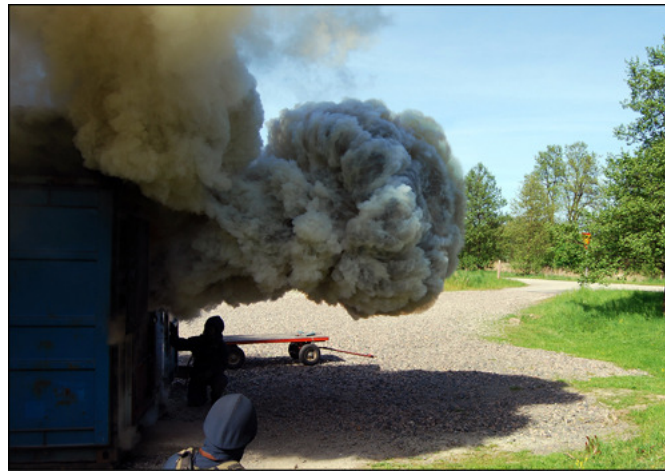
Figure 11 The excess pyrolyzates are pushed out through the opening. They will be ignited by the front of flames that is travelling towards the opening as well. This will result in the fireball that is typical for a backdraft. (Picture: Ed Hartin [20])
