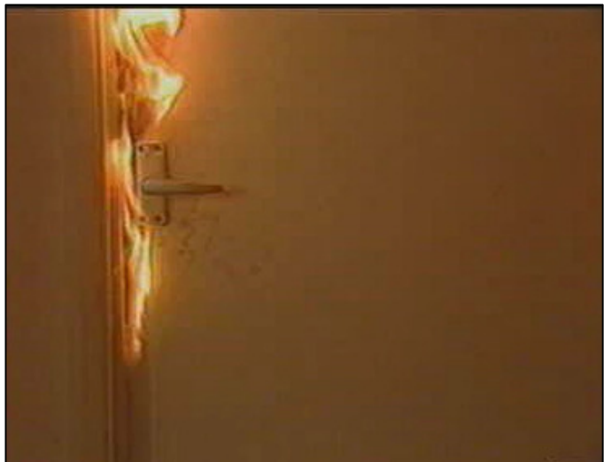
Figure 13 The smoke that is pushed through the gap is so hot that it auto-ignites at the outside of the compartment. This indicates an overpressure inside the room and the presence of a fire that is or has been very intense.
