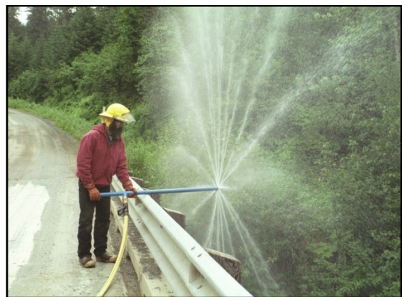
Figure 16 A piercing nozzle that disperses its water droplets radially (Picture: John Norman)
