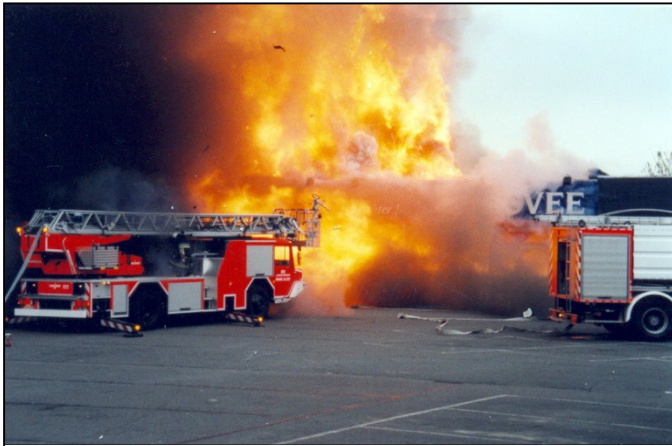
Figure 23 Backdraft after making an opening in the glass wall. (Picture: Benoît Amans)
