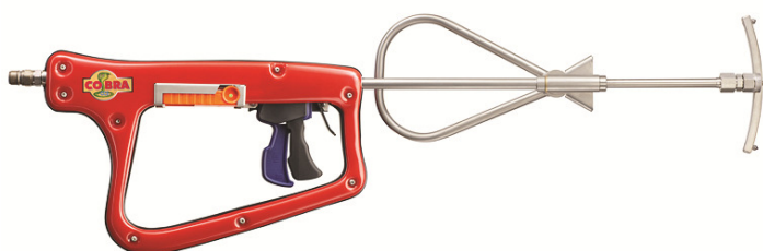
Figure 18 The Cobra nozzle. When both the triggers are pulled, both water and abrasive flow through the line. When only the blue trigger is pulled, only water flows. The orange block is the radio transmitter that sends signals to the pump. (Picture: Cold Cut Systems Svenska AB)
