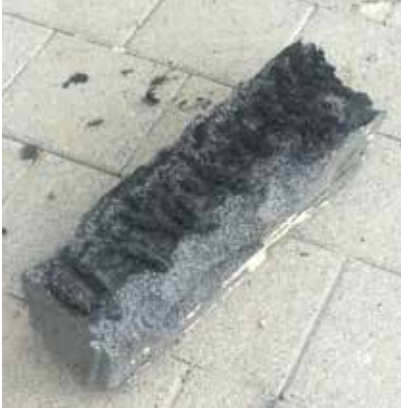
The partially burned EPS insulation. The upper part was smoldering and had blackened. Photo by Pieter Maes
